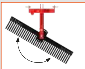
Up to 32° angling on standard duty rakes
