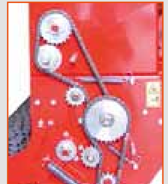
Seed distribution engaged by ASA 50 chain transmission
