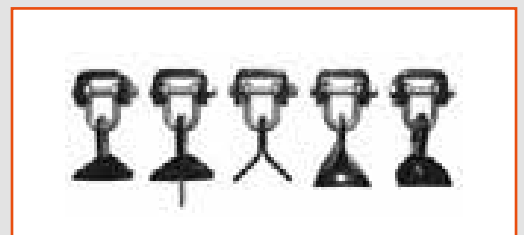
Choice of fine cut blades, detaching blades, reverse Y blades, paddle blades or hammer type blades
