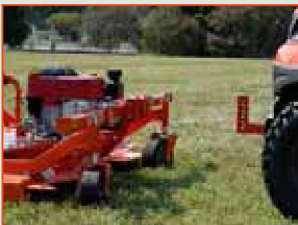
Front mount application with 2" receiver hitch
