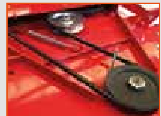
Heavy duty reinforced belt (BX) with automatic belt tensioner
