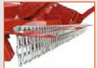
Chains provide safety from thrown objects
