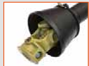
Driveline with shear pin safety
