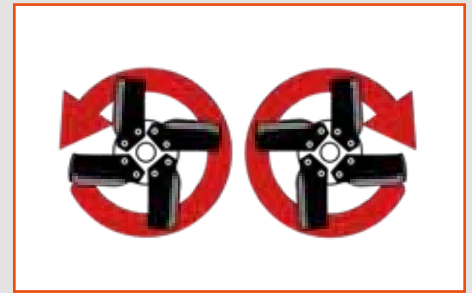
Forward or reverse tilling rotation
